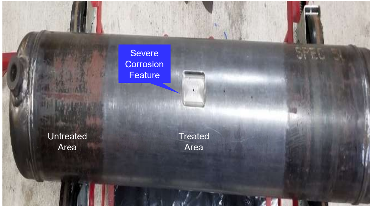
Figure 4. Pipe with PB 7000-M ONLY surface preparation with severe corrosion feature
