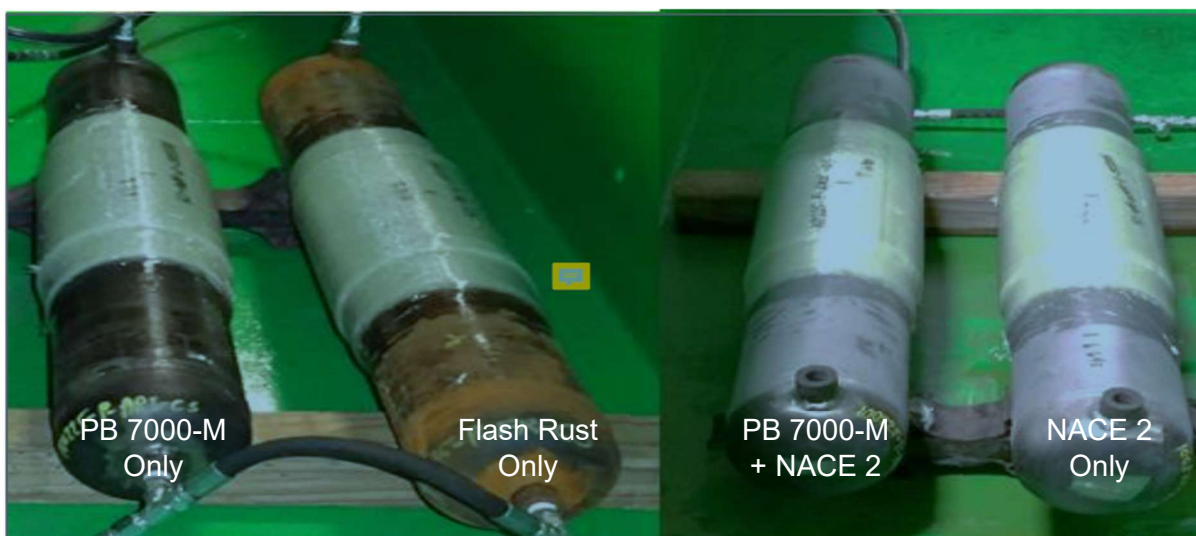
Figure 5. Pressure cycle testing of hybrid composite/steel sleeve repaired pipes
