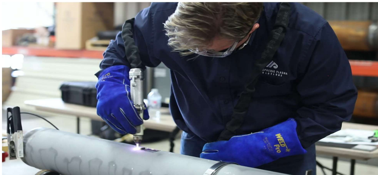
Figure 1. Using the PlasmaBlast™ 7000 Mobile System to conduct precision surface preparation on a pipe defect
